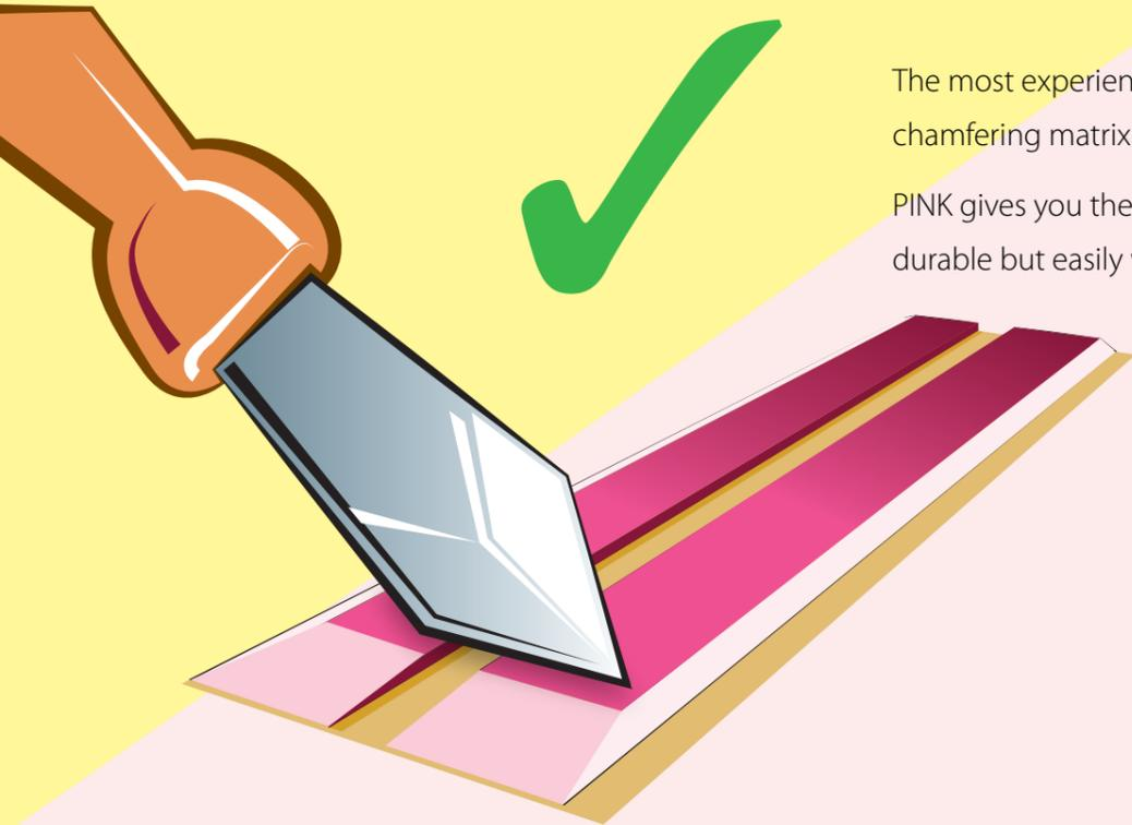
The most experienced operators will be used to chamfering matrix with a knife or sandpaper.
